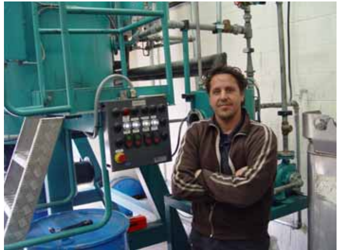
Evan Bradley (pictured here) with the Renzmann solvent recovery machine, which he installed after his NZCTF overseas training trip. The new machine is enabling the Convex printing department to clean, recycle and reuse solvents with minimal mess and downtime. It is also allowing Convex to do all their solvent recovery on site and has significantly reduced the team's exposure to solvents.
